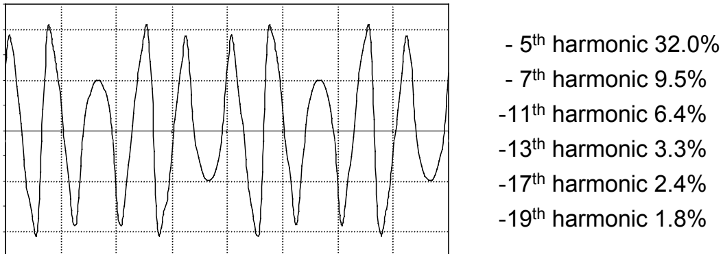
Figure 4. Current of an active filter and its harmonic content
