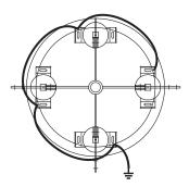
The diagram explains the manner in which earthing of equipment in the vicinity of air core reactors should be done. The overall principal is to avoid closed loops.
