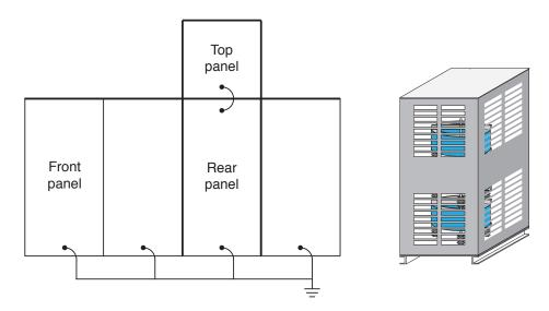
It is clear from the magnetic field plot presented at the start of this note that the highest magnetic flux density will exist directly above and beneath the reactor. In the case of enclosed reactors it may be beneficial to construct the top of the enclosure from a material such as fibreglass and to leave the bottom open.
