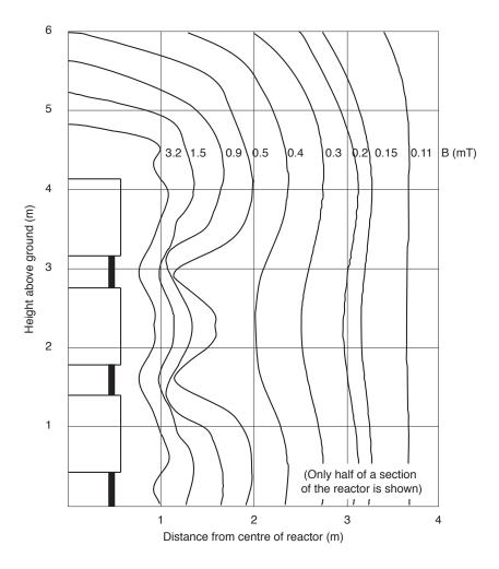
The analysis software takes into account the geometrical arrangement of the reactors and winding details. As an example it considers the impact of the vertical arrangement and the fact that in the
