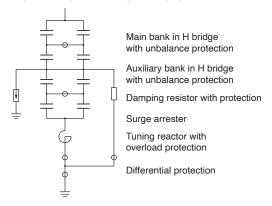
C-type filters have become ubiquitous in renewable generation projects for good reasons: excellent suppression of harmonic distortion across a wide range of frequencies (achieved by careful selection of tuned frequency and damping characteristics), low power frequency losses, small footprint, and relatively low cost when compared to alternative harmonic mitigation methods.
