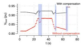
The statcom ensures that voltage variations are limited to well within the  $\pm 5\%$  range limit set by the network owner, under all load contingencies. The graph below illustrates how the statcom reactive power output changes instantaneously to ensure voltage levels are maintained.
