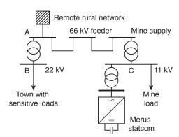
A statcom solution is supplied and connected to the mine's 11 kV busbar. The statcom consists of  $\pm 4$  Mvar of dynamic compensation and a 3.9 Mvar fixed capacitor bank. The performance of the solution is evaluated on the basis of a series of worst-case events: starting and stopping the large variable speed mill drives, starting the largest direct-on-line motor in the mine, and complete load rejection of the mine as a result of 66 kV breaker operation.
